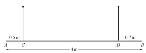
A beam, AB, has length 4 m and mass 20 kg. The beam is suspended horizontally by two vertical ropes. One rope is attached to the beam at C, where AC = 0.5 m. The other rope is attached to the beam at D, where DB = 0.7 m (see diagram).
