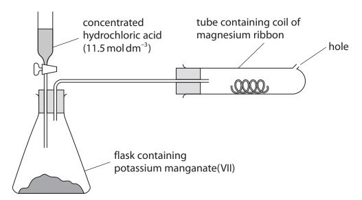
The coil of magnesium ribbon is first heated strongly until it just melts. Chlorine gas is then produced by a chemical reaction in the conical flask.
