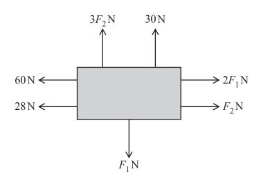
A body remains at rest when subjected to the horizontal and vertical forces shown in the diagram.
