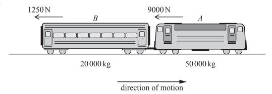
A train consists of an engine A of mass  $50\,000\,\mathrm{kg}$  and a carriage B of mass  $20\,000\,\mathrm{kg}$ . The engine and carriage are connected by a rigid coupling. The coupling is modelled as light and horizontal.
