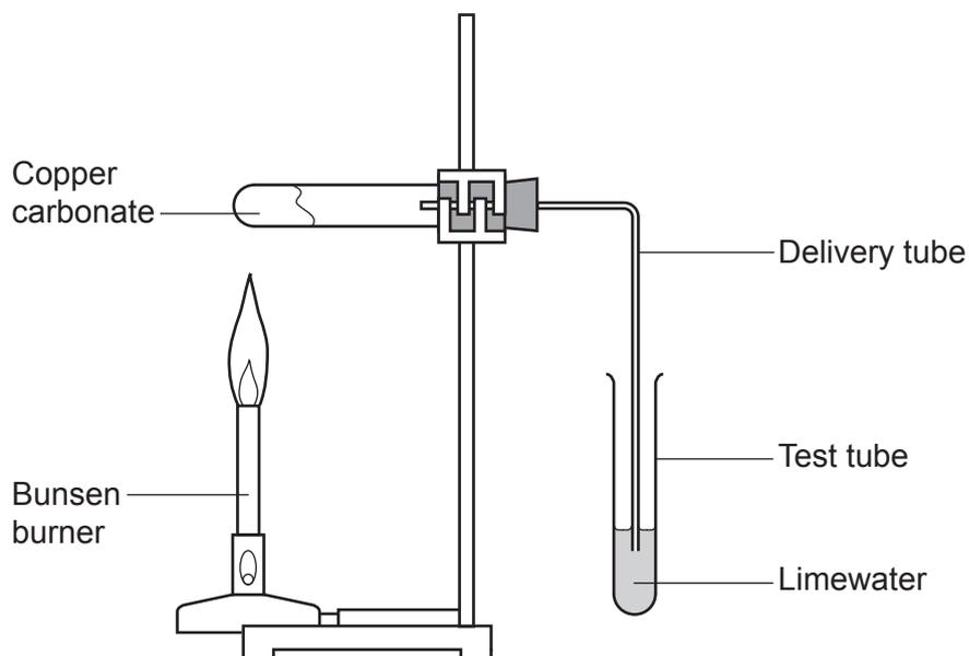
The student measures the mass of copper carbonate at the start of the experiment. She then measures the mass of copper oxide made.
